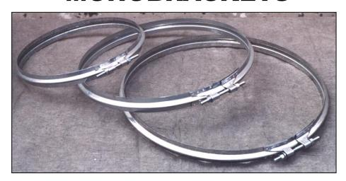
Constructed in zincated printed sheet. Thickness 8/10 from Ø 170 to Ø 500 Thickness 10/10 from Ø 510 to Ø 1500 Available by request in stainless steel.
