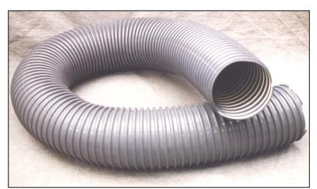
Flex pipe in plastic-coated PVC with reinforcement spiral in hard shock-resistant PVC. Suitable for AIR and SMOKES suction. Good resistance in suction. Employment temperature: -15° +60° C.
