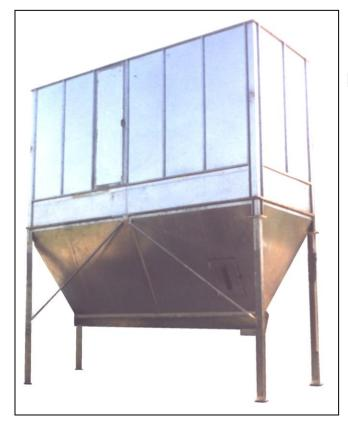
Handled filter sub-station employed for the suction and the filtration of wood shavings and dust.
